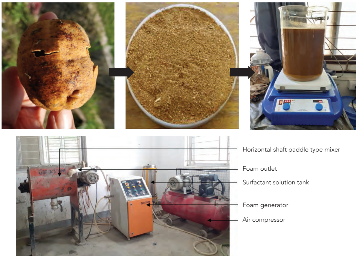
Figure 2: (a) Hingot fruit; (b) Pulverized hingot powder; (c) Hingot solution heated on hot plate magnetic stirrer; (d) Foam concrete production setup
