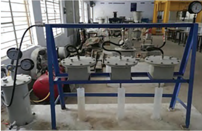
Figure 2: Water permeability test set-up
